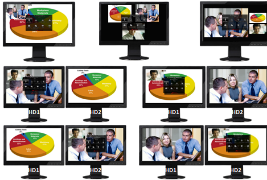
Figure 62: Examples of video layouts with three streams on single or dual monitors
